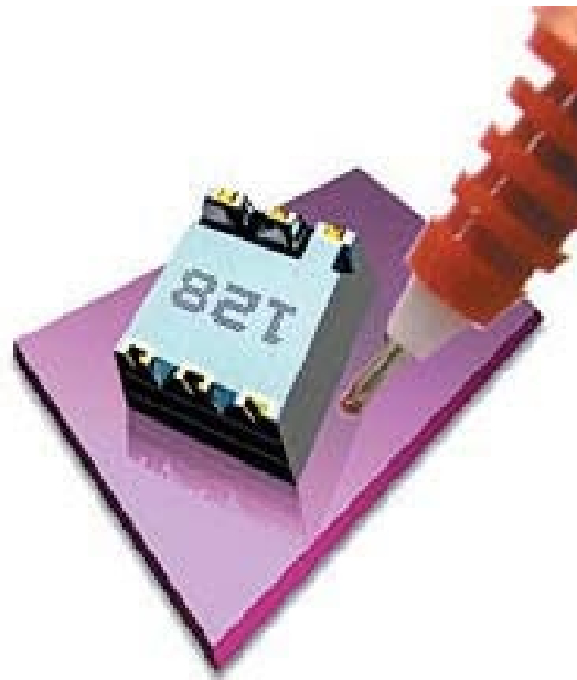
Photo1. The variable capacitance sensor element weighs 15 mg and measures 0.14 by 0.11 by 0.03 in high
