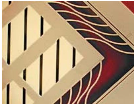
Photo 2. The beams in the suspension system supporting the inertial mass are typically 9 microns wide and 1.5 microns thick.
