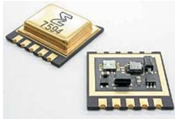
Photo 3. The Model 7594 OEM accelerometer is 5/8 by 5/8 in. with a height of 0.15 in. The weight is 1.6 g. The cover has been removed to display the sensor element and conditioning circuitry.
