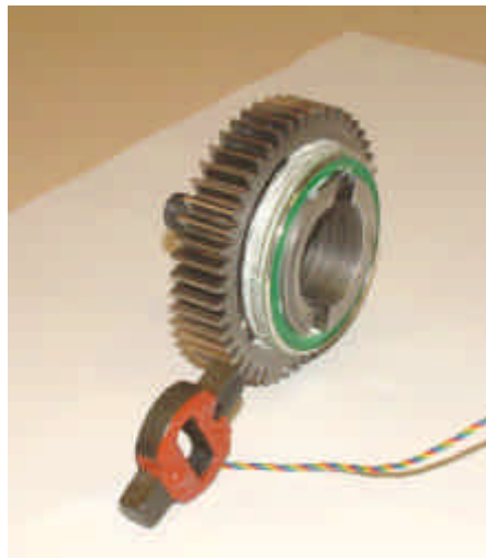
Fig. 1 Machined drive wheel and transducer.
